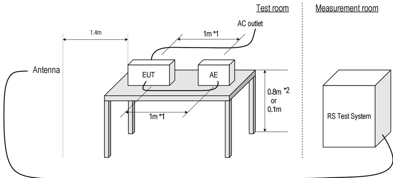
\*1: Wiring is left exposed to the electromagnetic field for a distance of 1m from the EUT.
