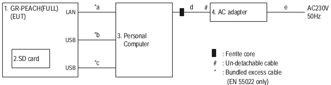
Note1: Numbers assigned to equipment or cables on this diagram correspond to the list in "3.1 Equipment(s) used" and "3.2 Cable(s) used".
